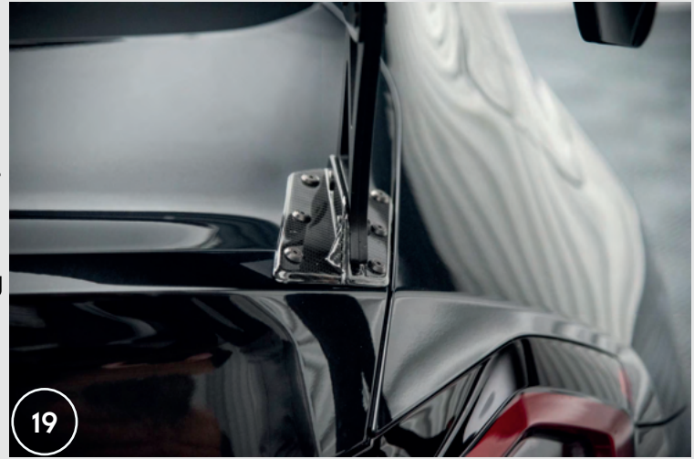
19. Place the spoiler mounting brackets with the trunk lid attachment and insert the threaded screws into the holes.
