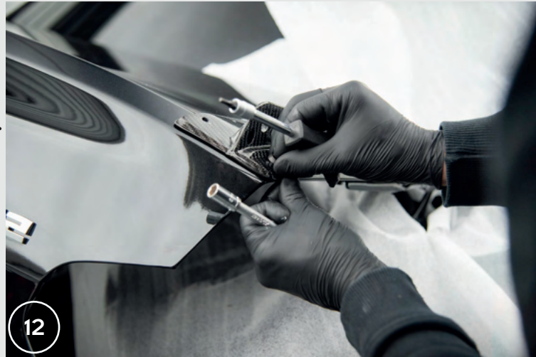
11. Prepare the mounting screws and washers. Apply a low-tear locking adhesive to the thread.
