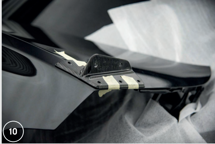
10. Secure the trunk lid mount with tape.
