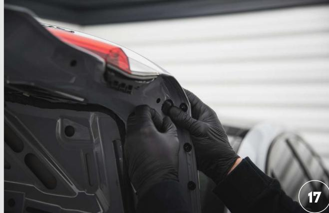
15. Screw the spoiler mount together with the seal to the trunk lid.
