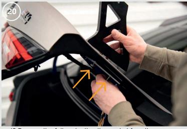
19.Remove the foil protecting the gasket from the lower part of the bracket.
