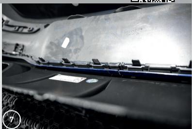
6. The mounting lugs should be visible from the inside of the bumper.
